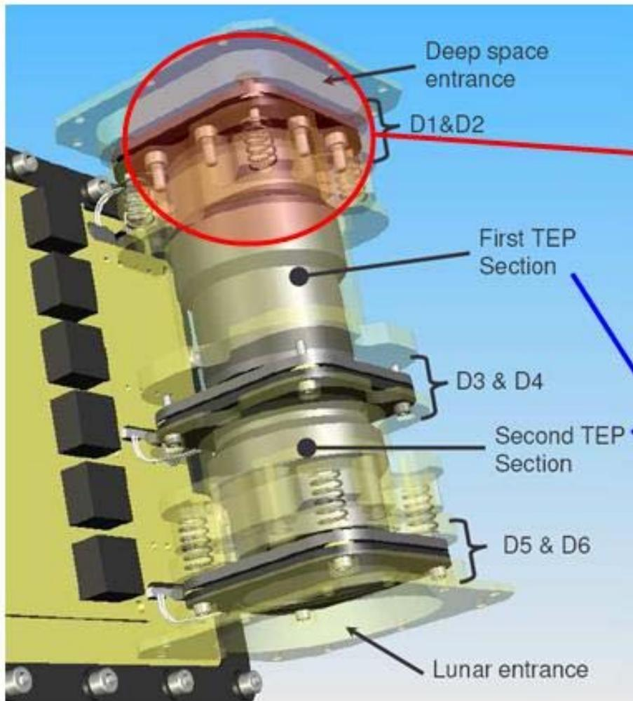
Pairs of thin and thick Silicon detectors
