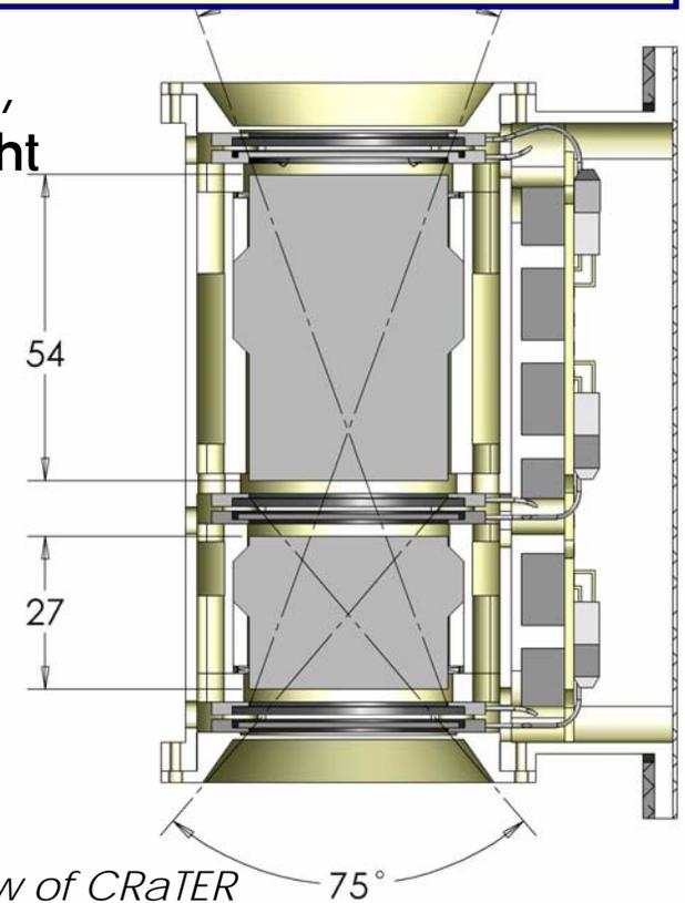
*Cutaway view of CRaTER*
